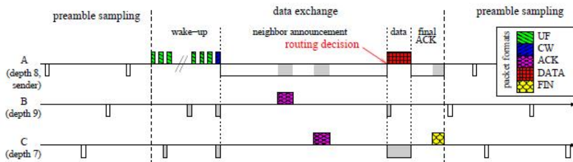
Figure 7.1: Timeline illustrating the execution of the protocol stack. The x-axis represents time; a box above the line indicates that the radio is transmitting; a gray/white box under the axes means that the radio is receiving/idle listening, resp.; no box means the radio is turned off.
