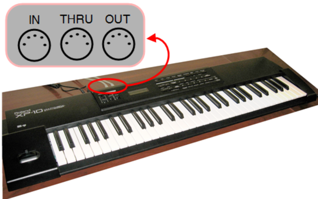
Figure 1.1: Rear-panel MIDI connectors for IN, OUT, and THRU
