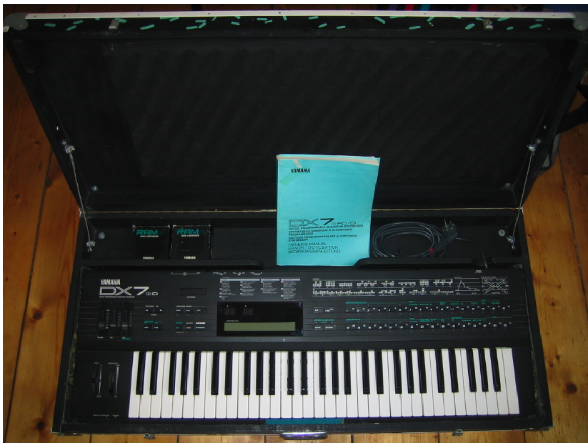
Figure 4.1: Yamaha DX7 synthesizer, the first commercially successful instrument to offer FM synthesis, digital synthesis, and MIDI compatibility. The instrument pictured here is packaged in a road case. Photographer: schoschie ( http://www.flickr.com/photos/schoschie/51653026/ 5 ). Copyright holder has granted permission to display this image under the Creative Commons Attribution-ShareAlike license 6 .
