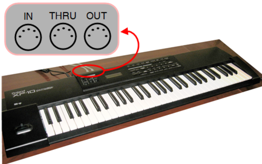
Figure 4.1: Rear-panel MIDI connectors for IN, OUT, and THRU
