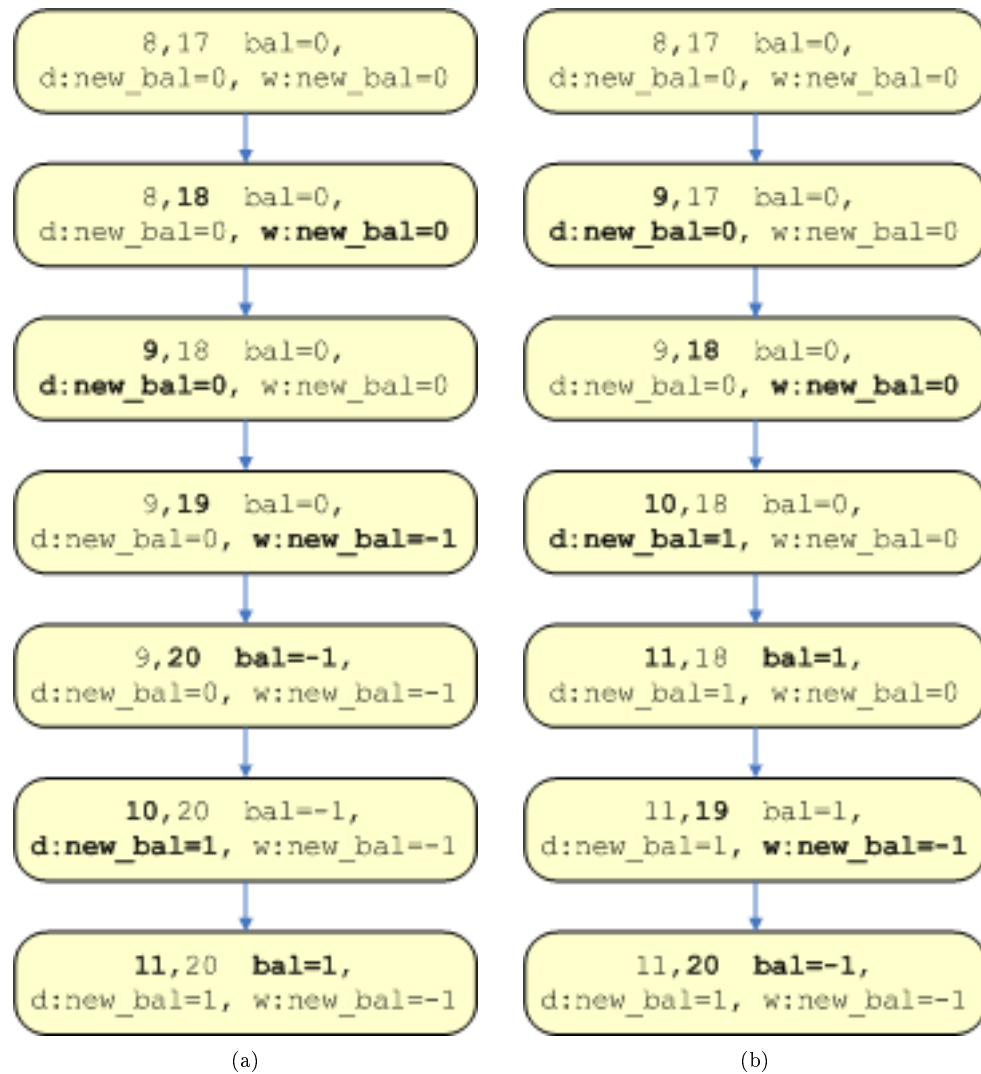
Figure 4.10: Two possible traces for the above program resulting in undesired non-zero results.
