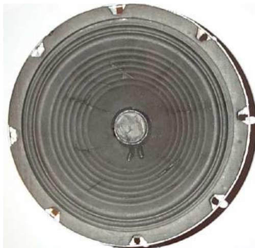
Figure 3.10: Mishandled driver with additional cuts in the cone
