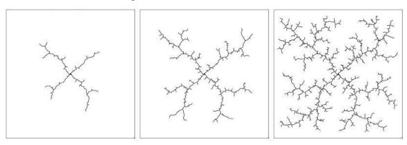
Figure 8: Tree-based planners start at a point and grow outwards, covering the configuration space more and more densely as time goes on.
