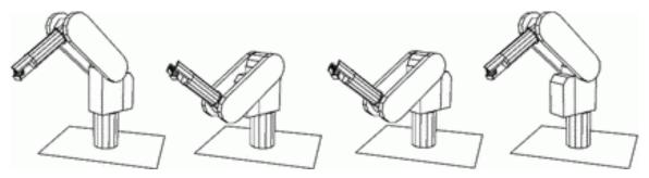
**Figure 2:** The spatial constraint on the end-effector of this three-dimensional manipulator can be satisfied by a maximum of four different configurations of the manipulator. Figure is obtained from Serial Robots <sup>44</sup>.
