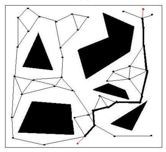
Figure 7: The start and goal configurations are connected to their nearest neighbors in the roadmap. A graph search is then made to find the shortest path in the roadmap from start to goal.
