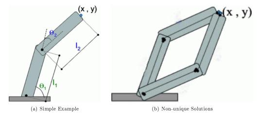
**Figure 1:** Illustration of solving the Inverse Kinematics problem for a simple planar robot with two arms. Figure is adapted from MathWorks<sup>43</sup>. (a) Steer end-effector to (x, y) target position. (b) Two solutions depicted for this IK problem.
