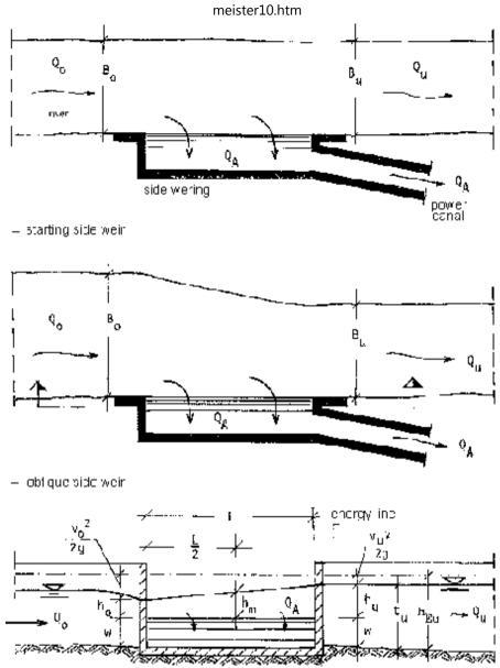
Fig. 36: Principle of the side weir with the hydraulic characteristics.  $Q_0$  headwater discharge,  $Q_u$  tail water discharge,  $Q_A$  evacuated amount of water, w weir height, L weir length,  $h_0$  weir head in the headwater,  $h_u$  weir head in the tail water,  $h_m$  mean weir head,  $h_{Eu}$  energy head in the tail water,  $v_{0,u}$  flow velocity in the headwater, tail water
