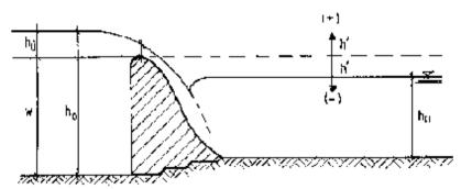
Fig. 34: Discharge over a weir
