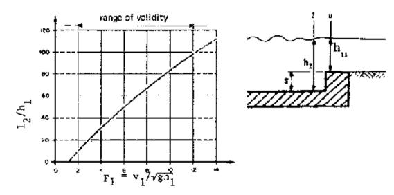
Fig. 4: Diagram for determining the hydraulic jump length I<sub>2</sub> for horizontal rectangular
