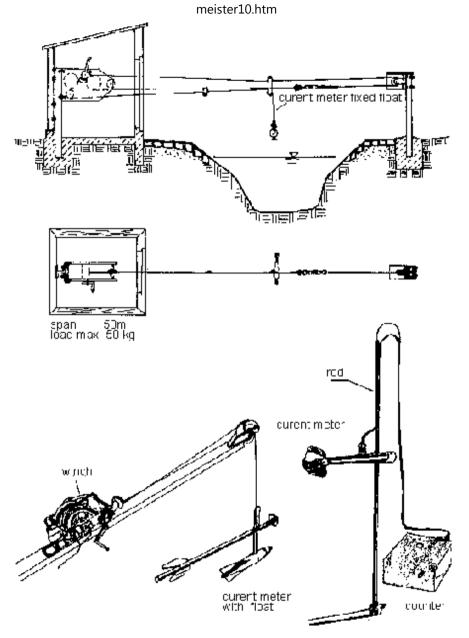
Fig. 5: Discharge measuring instruments for current meter measurement
