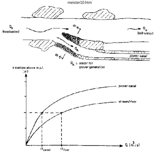
Fig. 39: Lateral intake with repelling groin
