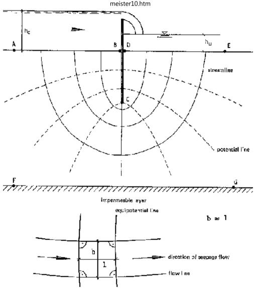
Fig. 41: Construction of a stream and potential line net
