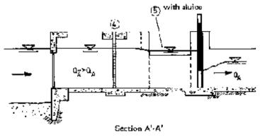
schematic, ongitudinal section through an inlet structure
