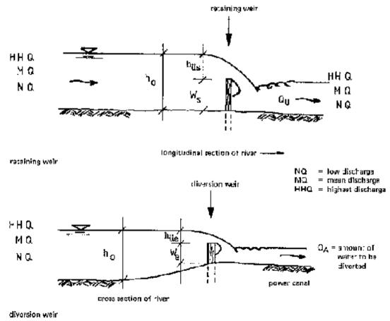
Fig. 35: Relationship between diversion weir and retaining weir
