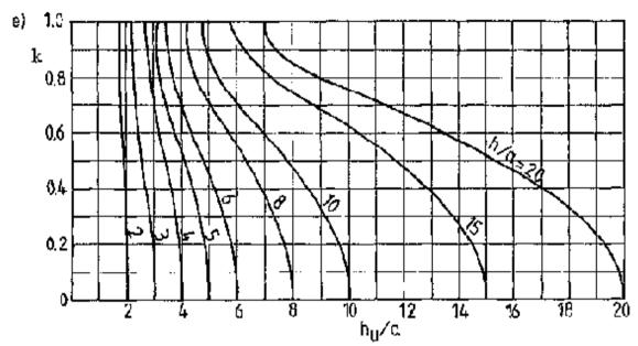
Fig. 38: Dimensioning of the discharge below a sluice,  $\delta$  contraction coefficient
