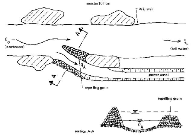
Fig. 29: Simple intake structure without damming with repelling groin
