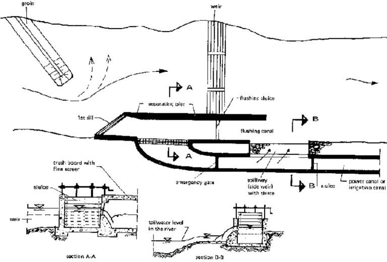
Fig. 28: Intake structure with bed load removal (flushing canal) and spillway (side weir)
