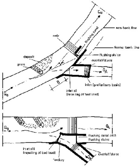
Fig. 18b: Lateral intake with damming and repelling of bed load from intake by technical measures
