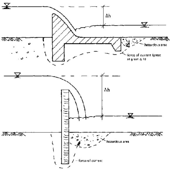
Underflow of structures; zones subject to danger of hydraulic shear failure
