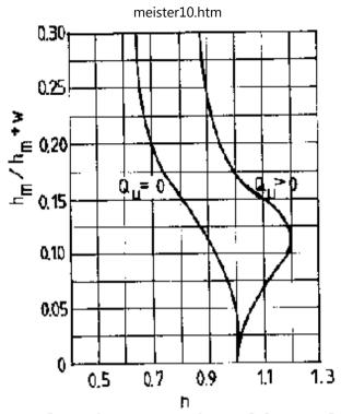
Fig. 37: Correction factor n for side weir calculation
