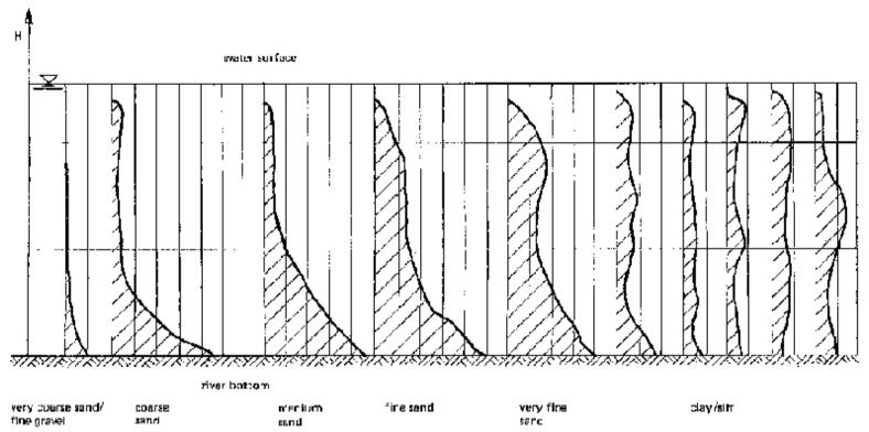
Fig. 15: Distribution of suspended matter concentration of various soil types
