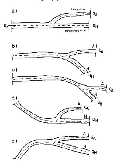
Fig. 17b: Entry of bed load in lateral intakes without additional structures according to [6]
