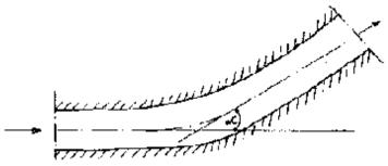
Fig. 19: Angle of bend  $\alpha$ Slight bend at a < 30°
