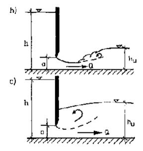
Fig. 38: Dimensioning of the discharge below a sluice, a contraction coefficient
