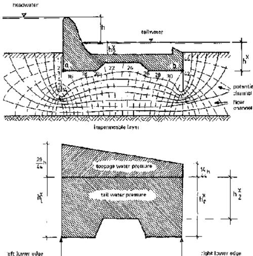
— Number of potantial fines n<sub>a</sub> = 44 (numerical example)
