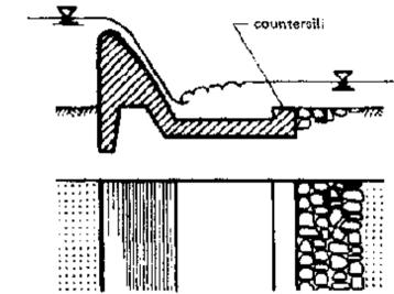
Fig. 3: Stilling basin with countersill
