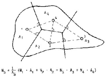
Fig. 10: Thiessen polygon method for the determination of the precipitation area
