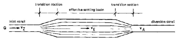
Fig. 44: Schematic representation of a uniformly loaded sand trap
