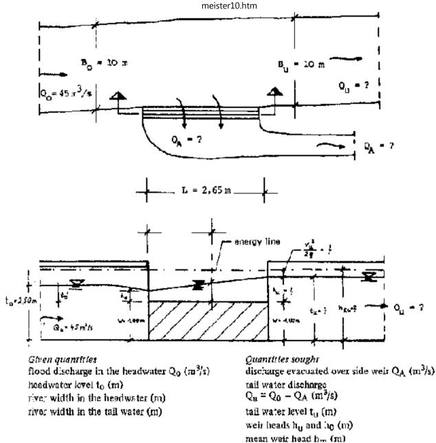
Fig. 1: Overfall over a straight side weir - flood event (numerical example)
