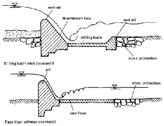
Fig. 21: Elements of a fixed weir
