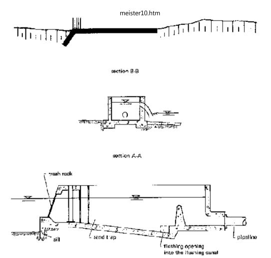
Fig. 27: Intake structure for a small hydroelectric power plant with sand trap and bed load removal (flushing canal) - basic sketch
