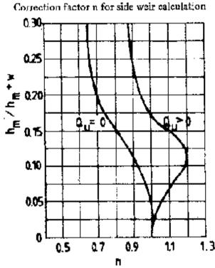
Correction factor n for side weir calculation
