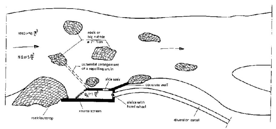
Fig. 30: Lateral intake without damming - basic sketch
