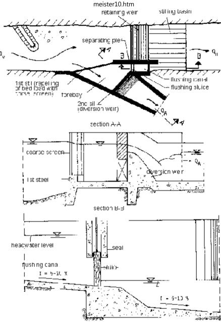
Fig. 26: Example of an intake structure and flushing canal for bed load removal (QA > 0.5  $\cdot$  Q0) - basic sketch
