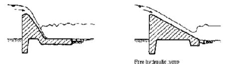
Fig. 2: Dammed hydraulic jump; Free hydraulic jump
