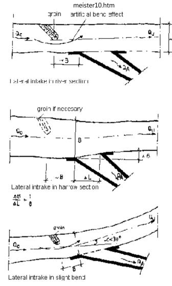
Fig. 18a: lateral intake without damming and repelling of bed load from intake by technical measures
