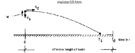
Fig. 45: Longitudinal section of sand trap. Schematic path curve of a settling sand particle "K" under the influence of turbulence.  $v_d$  flow velocity in the basin,  $v_s$  sinking velocity in stagnant water, w dynamic buoyancy due to turbulent flow; condition:  $t_d$   $^3$   $t_s$
