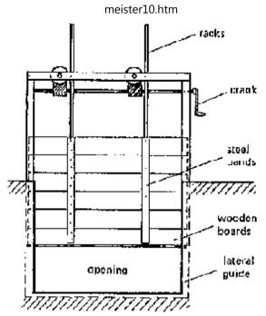
Fig. 25: Sliding sluice
