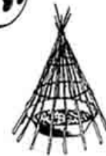
wooden feeder - top bar supported by two nails, moves round if chickens try to jump on it
