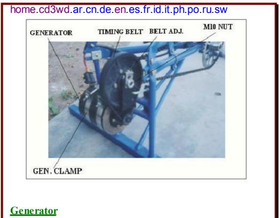
It is a permanent magnet DC generator. Suitable for 12 volt batteries
