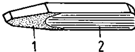
Figure 2 – Cut through a hardened chisel – 1 cutting edge (hard), 2 twig (tough)
