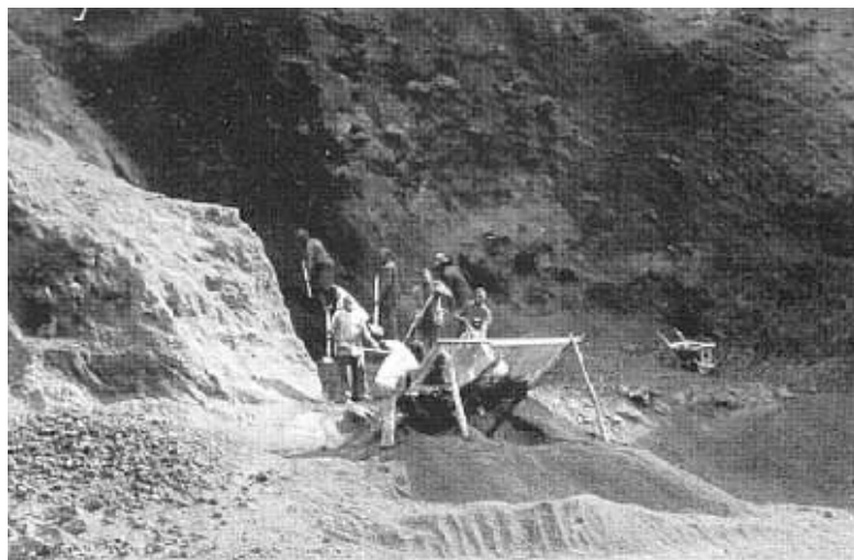
Figure 2: Volcanic ash pozzolana being excavated – Rwanda.
