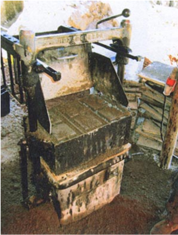
Removing the mould upwards
