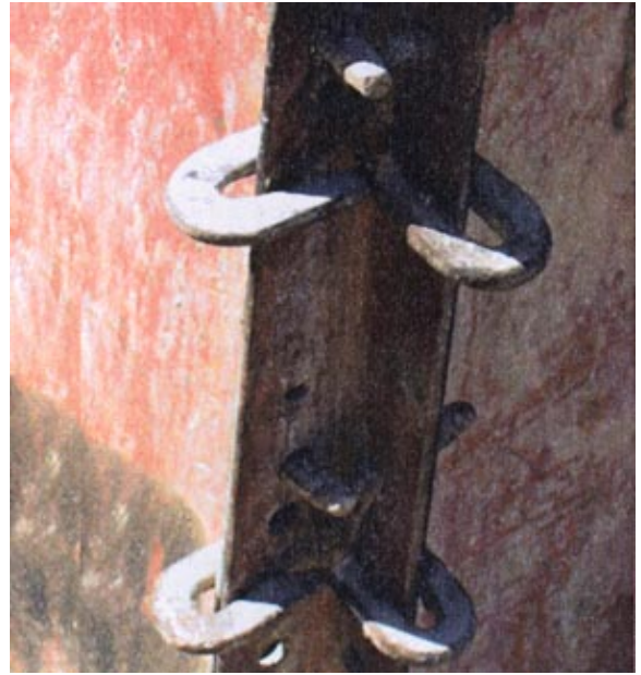
Four clamps mounted in edge-position using an angle bar
