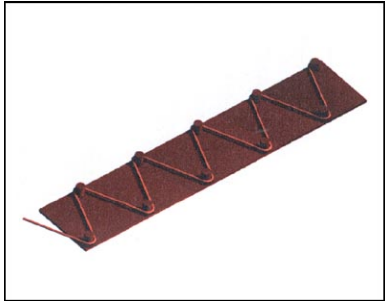
Model of the formwork with ready-bent stirrup on it
