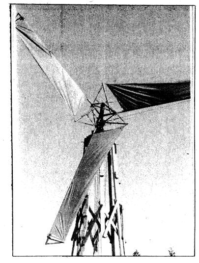
of a village wheel wright cum blacksmith are required for production of the oxcart wheel and mounting the wheel on the turntable shaft, the sails are manufactured on a standard sewing machine. The occasional presence of one person is required for operation. The Windmill is intended for the direct use and operation by its owner-builder.
