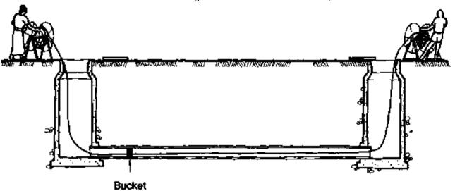
Fig. 27. Cleaning of closed drains using a bucket
