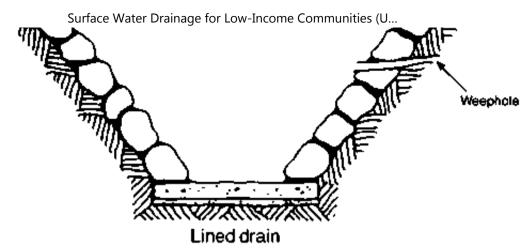
Fig. 11. Cross-sections of typical unlined, partially lined and lined drains
