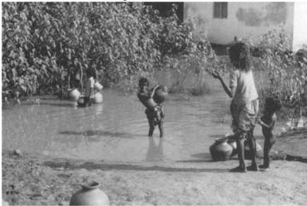
A public water tap in a poorly drained low-income community in Pondicherry, India. Sanitary services such as water supply and excreta disposal cannot function hygienically without adequate surface water drainage.
