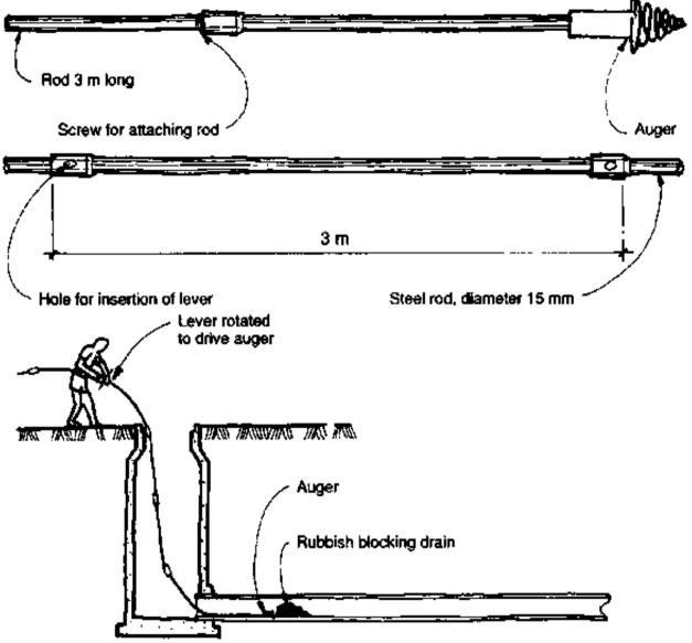
Fig. 28. Cleaning of closed drains using an auger
