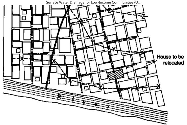
Fig. 20. Sketch for planning a drainage system
