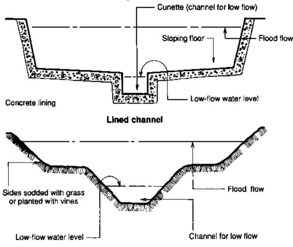
Unlined channel Fig. 9. Cross-sections of typical composite drainage channels
