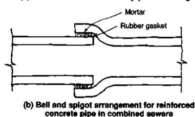
Fig. 16. Jointing of reinforced concrete pipes
