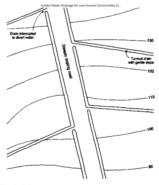
Fig. 5. Turnout drains to divert water from a steep slope
