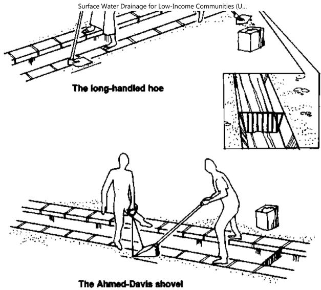
Fig. 26. Tools for cleaning drains
