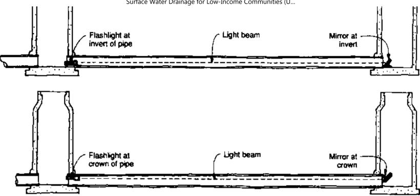
(a) Light is well aligned - light at one end is reflected by the mirror when placed at crown and invert
