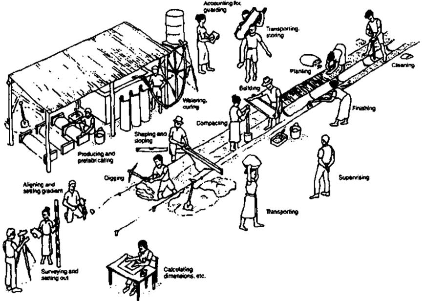
Fig. 19. Tasks in drainage construction
