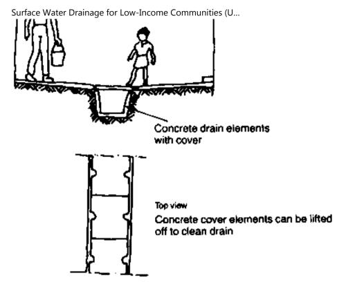
Fig. 13. Combined drains and pathways
