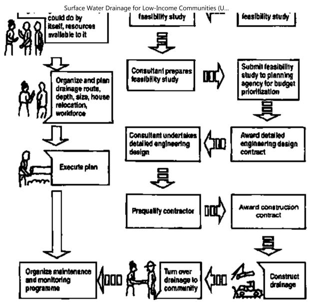
Fig. 4. Possible sequences of events in solving local drainage problems
