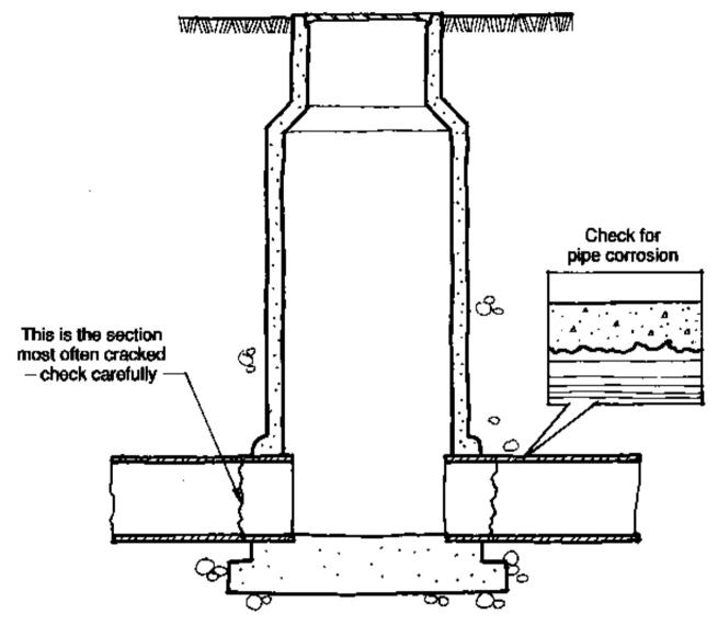
Fig. 24. Common failure sites in closed drains
