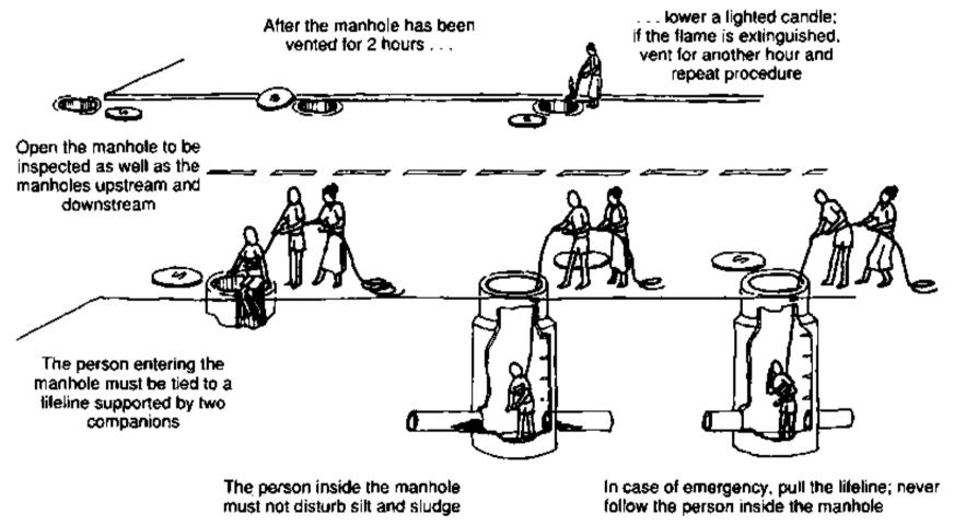
Fig. 22. Safety in entering closed drains
