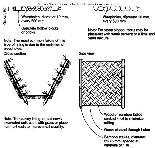
Fig. 12. Types of drainage channel lining
