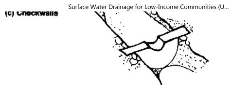
Fig. 6. Types of construction for steep drains
