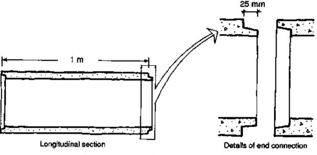
(a) Normal reinforced cement pipe for drainage
