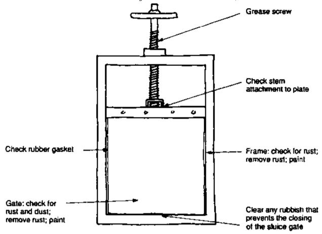
Fig. 25. Requirements for maintenance of sluice gates
